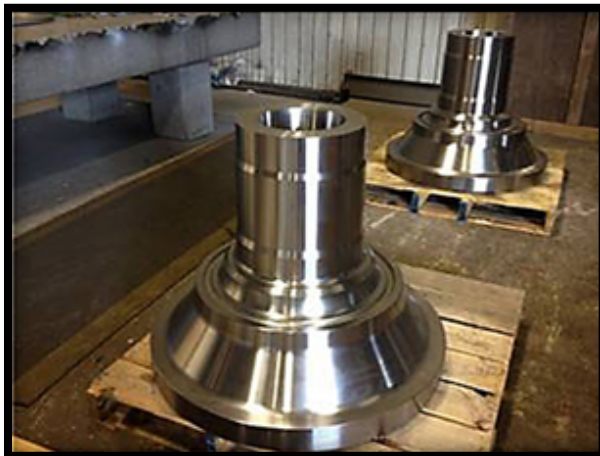
Spindles manufactured at Ellwood Texas Forge & Machine
